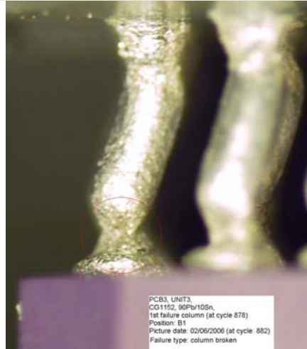
CG1152 90 Pb / 10 Sn, Cycle 882 1 st failure at cycle 878
