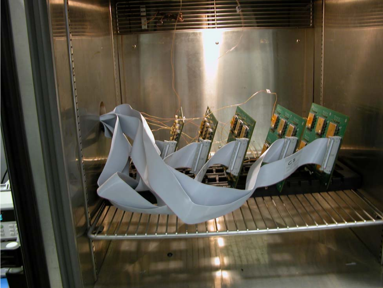
Figure 4: Testing PCBs in Oven
