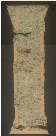
CG1152 80 Pb / 20 Sn, Cycle 1225 1 st failure at cycle 1212
